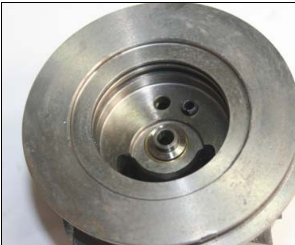
Then put the thrust ring on the right position
