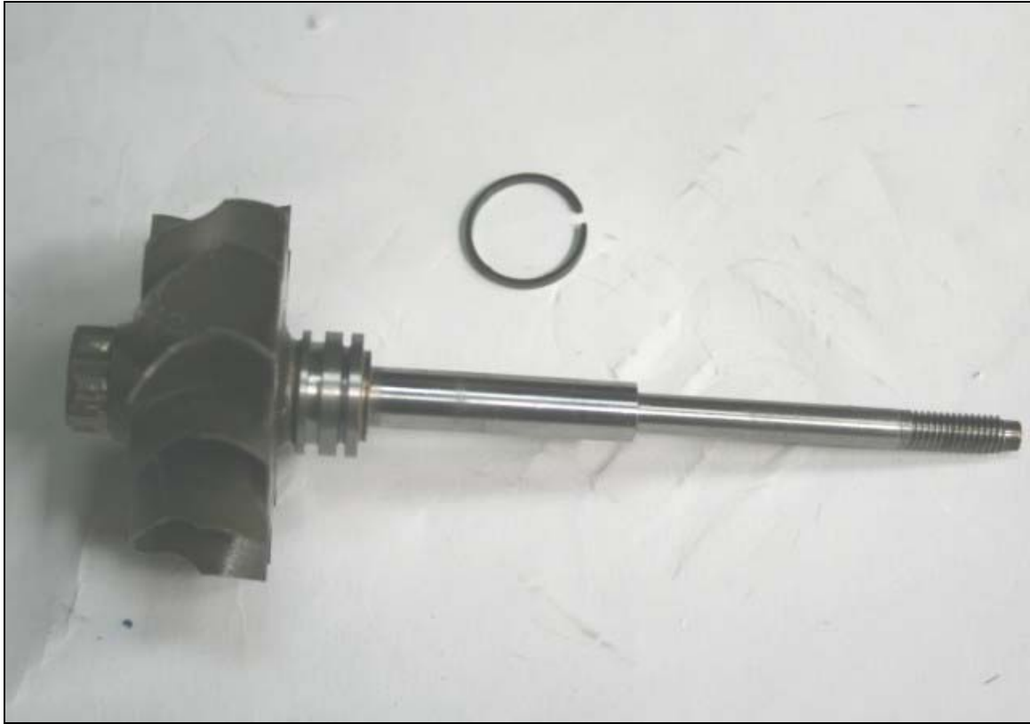
Here shows turbine shaft / wheel and new piston ring.
