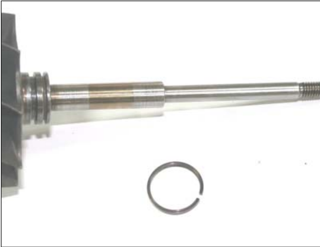
The pictures shows the turbine shaft after we clean carbon on the groove and shaft
