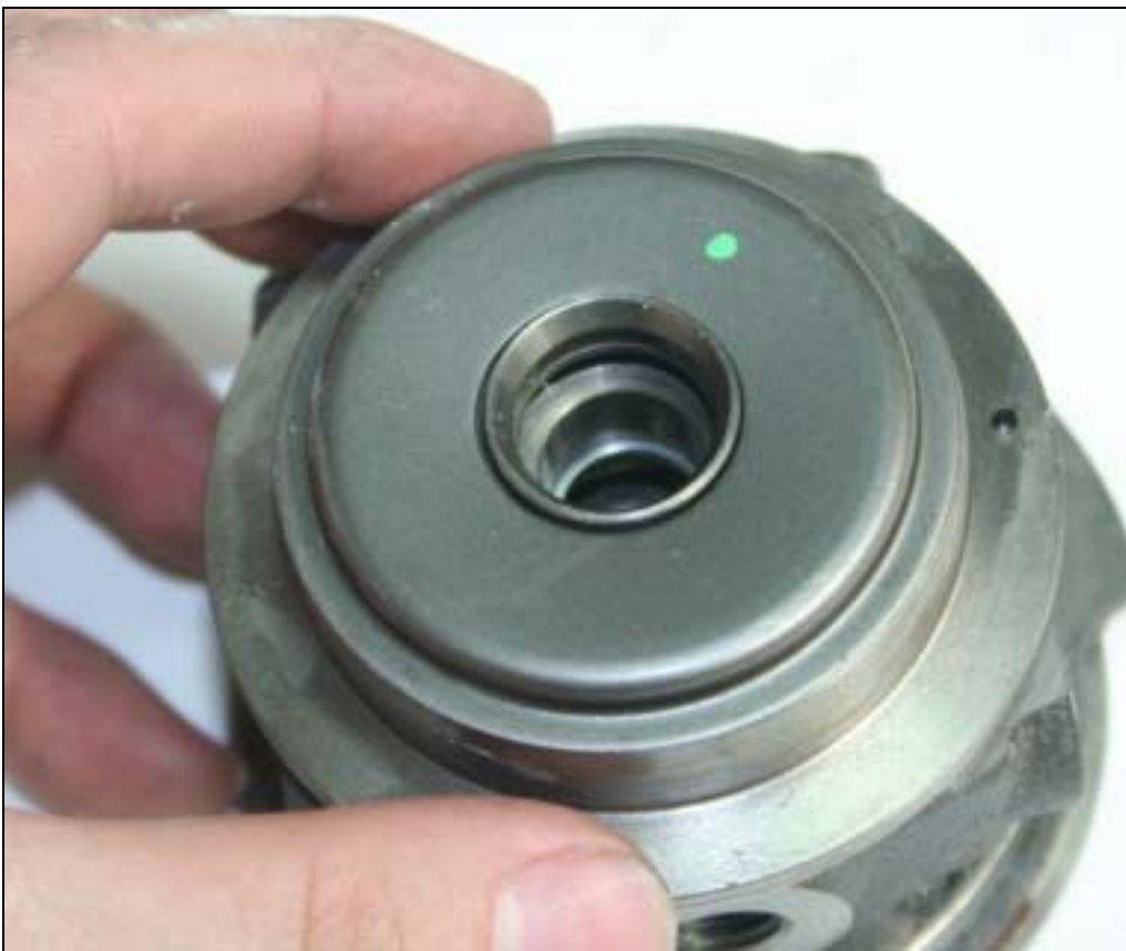
Place Heat shield on the bearing housing
