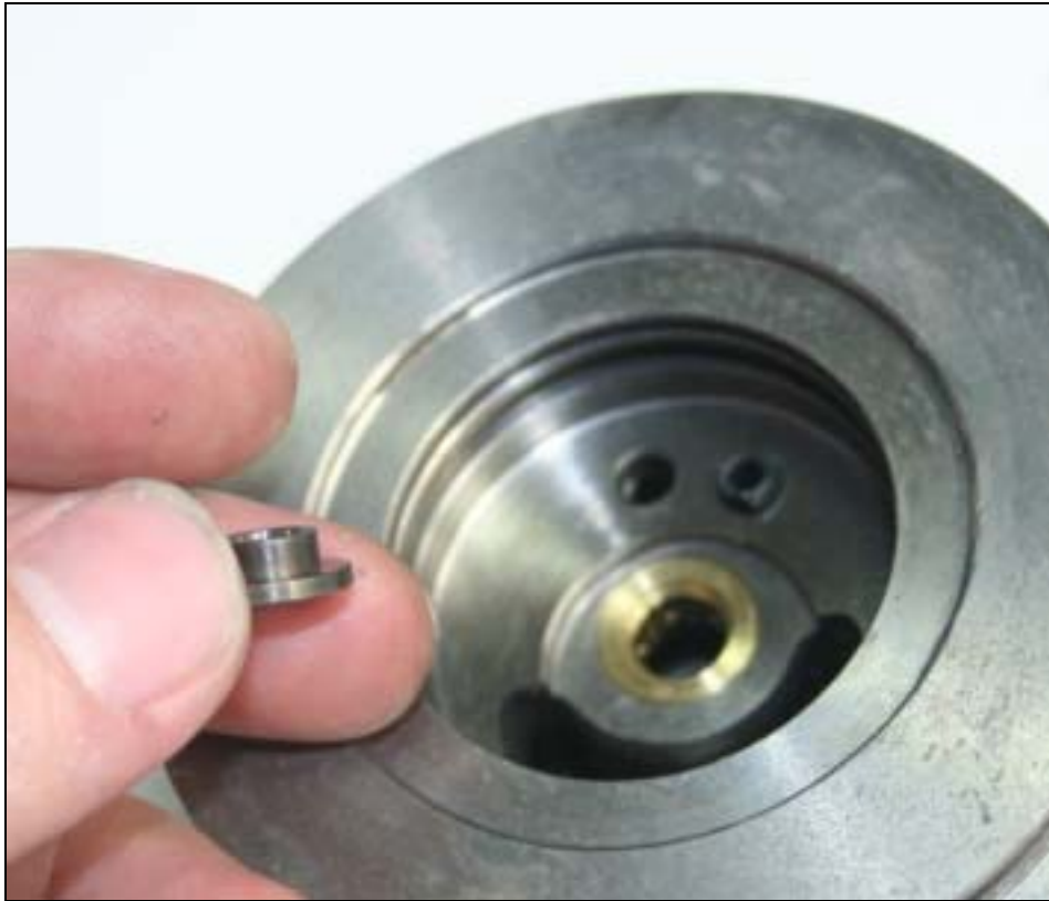
Then put the thrust ring on the right position
