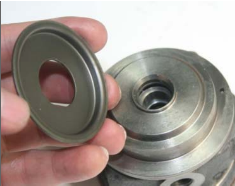
Place Heat shield on the bearing housing
