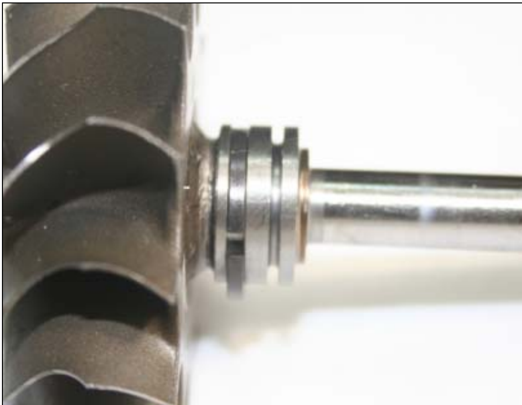
press the piston ring into groove
